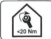
EXTERNAL CONNECTIONS FITTED TO THE CO<sub>2</sub> DISTRIBUTOR MUST NOT BE TIGHTENED WITH A TORQUE HIGHER THAN 20 Nm
